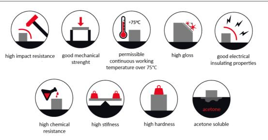
**ABS** is one of the key technical materials commonly seen in everyday life. That makes it widely popular in 3D printing as well, even though it is a bit more demanding than PLA. ABS stands out with remarkably high impact resistance, while retaining high stiffness, higher temperature resistance than PLA and ease of machining or chemical treatment. It's great choice when durability and toughness is the key.
